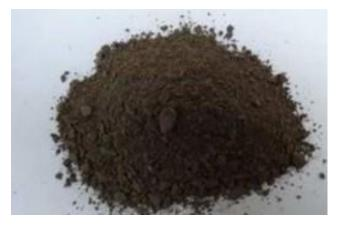
Fig. 3: Oil Shale Powder
