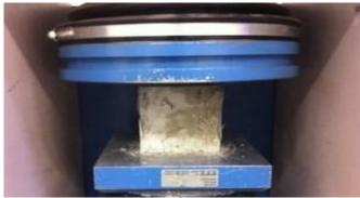
Fig. 6: Compressive testing machine
