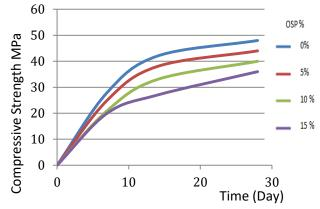
Fig. 7: Effect of binder OSP content and curing time on compressive strength (Mpa)
