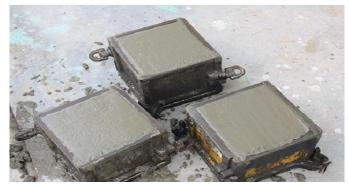
Fig. 5: Concrete Cubes (150x150x150 mm)
