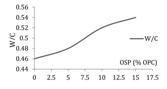
Fig 9 : Relation between OSP % in binder and the required water cement ratio
