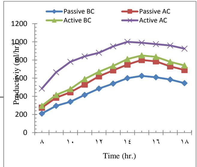
Figure 5: Daily productivity from the water depth of 0.5 cm. Another set of experiments was made to evaluate the effect of changing the water depth on the daily productivity. The same testing procedure was applied for each water depth; the obtained results from both modes of operation (Passive and Active) were recorded. Clear image regarding the obtained results from the Passive mode are presented in Figure 6, daily productivity as before and after cooling are clearly shown.
