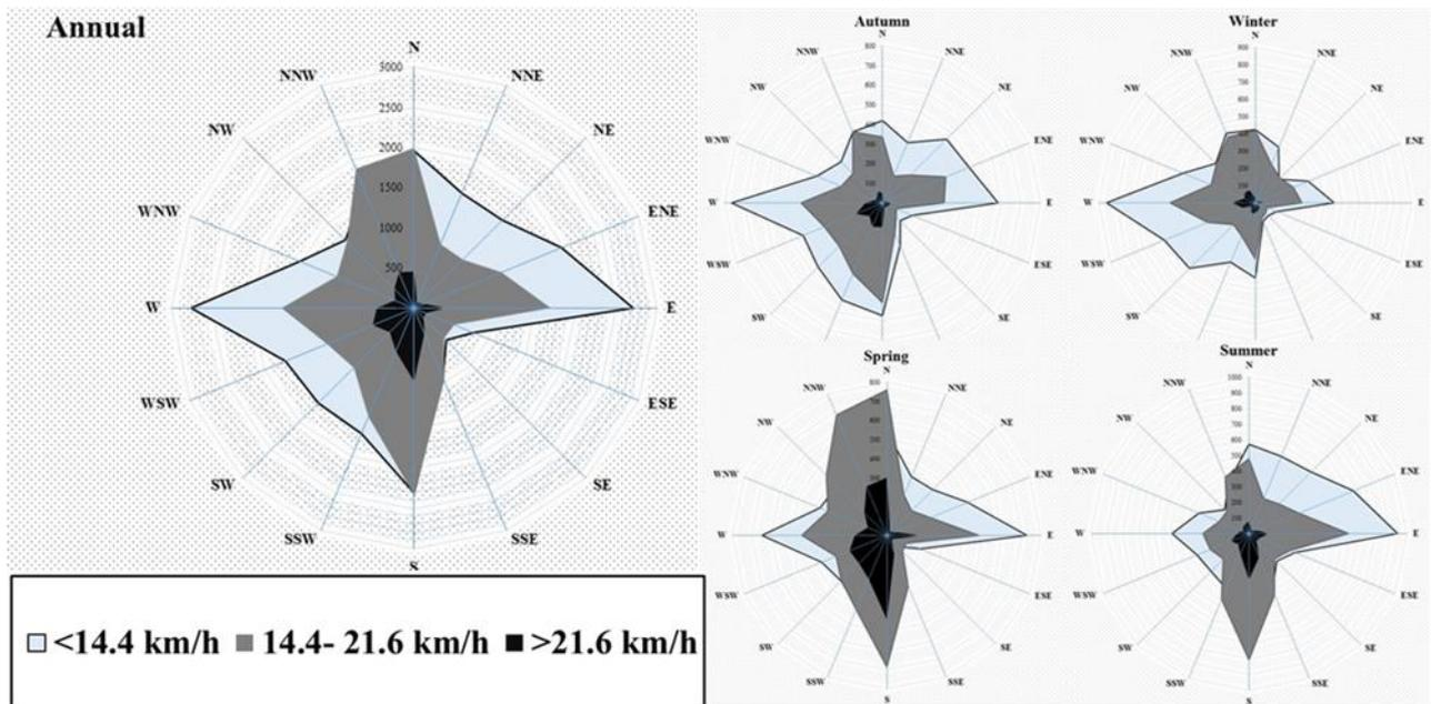
**Fig.03:** Wind rose diagram showing the directional and frequency variability of the all wind speed categories, from the station Ain sefra airport. Similar to the whole period: Annual and seasonal by observations of 1985-2015.
