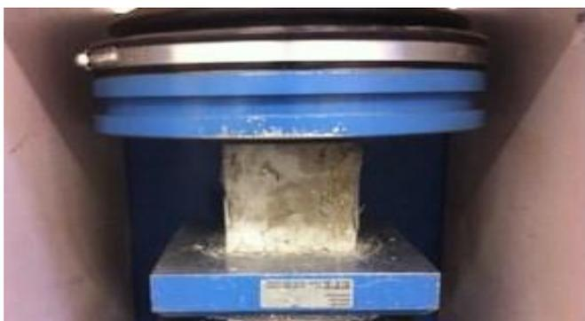
Fig. 6: Compressive testing machine
