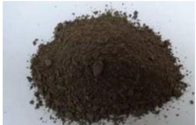
Fig. 3: Oil Shale Powder
