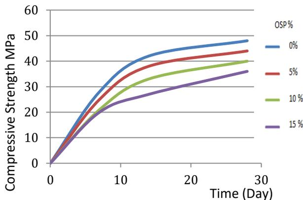
Fig. 7: Effect of binder OSP content and curing time on compressive strength (Mpa)
