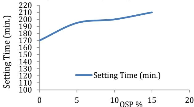
Fig. 8: Relation between the setting time and the ratio of OSP in binder
