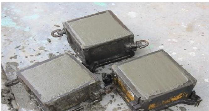
Fig. 5: Concrete Cubes (150x150x150 mm)
