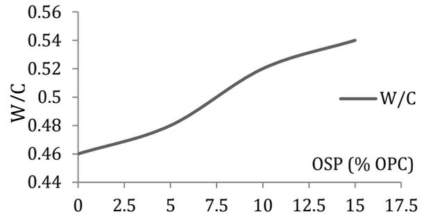
Fig 9 : Relation between OSP % in binder and the required water cement ratio
