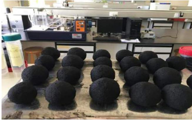
**Figure 8.** Pressed pyrolysis black carbon.
