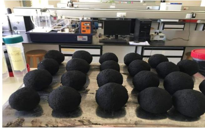
**Figure 8.** Pressed pyrolysis black carbon.
