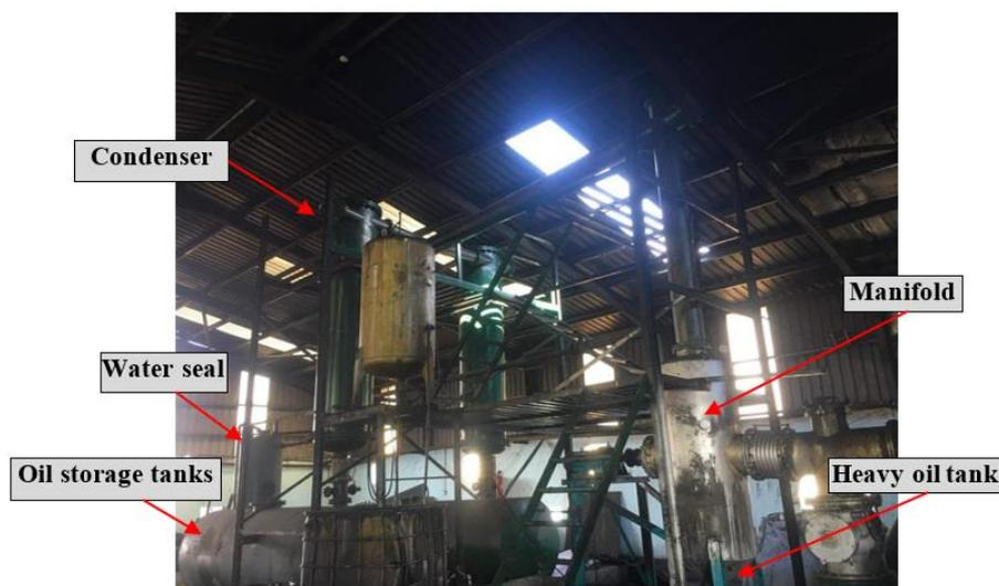
**Figure 4.** Manifold, heavy oil tank, condenser system, oil storage tanks and water seal.
