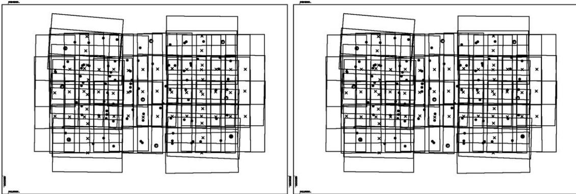
Figure 5. Block of 18 images taken at 1500m flying height (left) and block of image taken at 880m flying height (right) – using the UltraCam D
