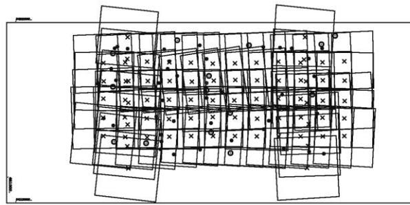
Figure 6. Block of photographs taken at 880m flying height – using the metric frame camera
