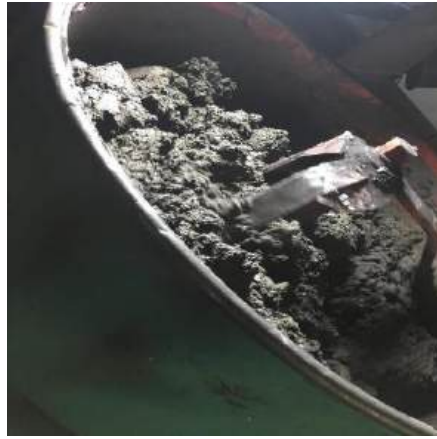
Figure 10. Mixing pyrolytic black carbon with gelatinized starch in Aqaba's tire pyrolysis industry.
