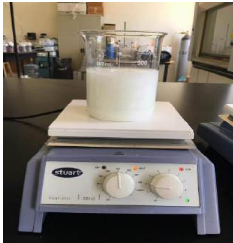
Figure 9. Starch is added to the room temperature water and start stirring it to dissolve before heating process.
