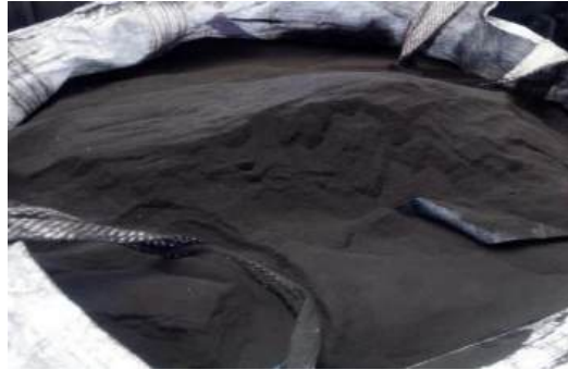
Figure 6. A sample of pyrolysis black carbon after pyrolysis process and before treatment.
